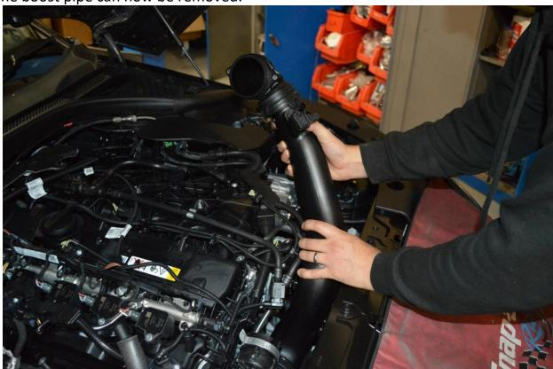
13. Remove the o-rings from both couplers on the boost pipe and place into the Forge hard pipe kit.
