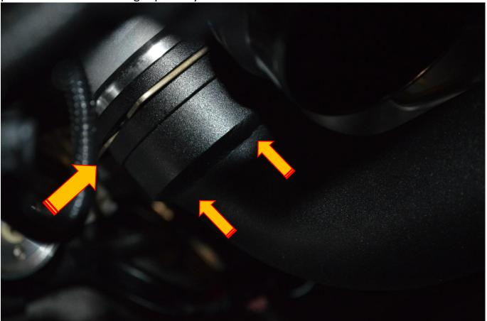
18. Place the silicone hose reducer into postion but do not fully tighten the hose clamps.
