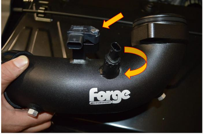
16. Ensure the water meth blanks are tightened fully.
