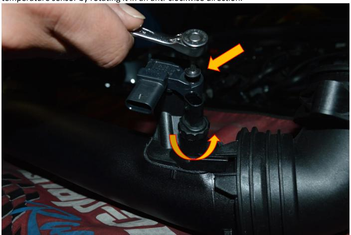
15. Fit the sensors into the Forge hard pipe using the fasteners provided.
