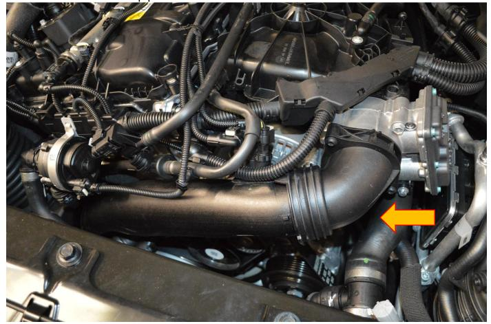
3. Disconnect the wiring loom to the pressure and air temp sensors on the boost pipe by depressing the grey tab and sliding outwards.
