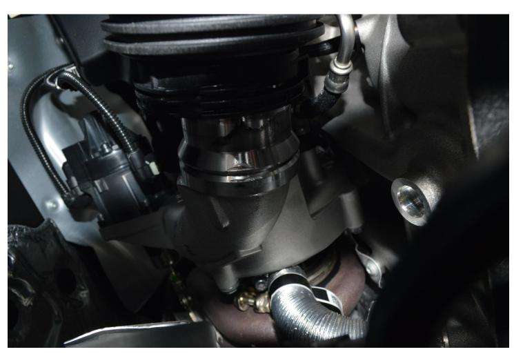
9. Remove the two retaining clips from the inlet pipe that joins to the turbo.
