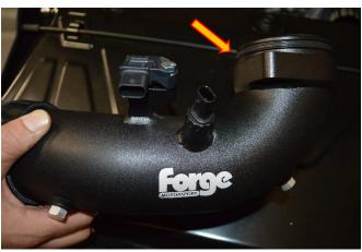
14. Using a T25 Torx drive, remove the boost sensor from the oem pipe, remove the temperature sensor by rotating it in an anti-clockwise direction.
