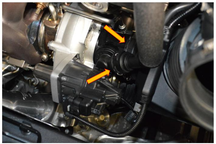
10. Remove the breather pipe from the inlet hose by depressing either side of the fitting while pulling.
