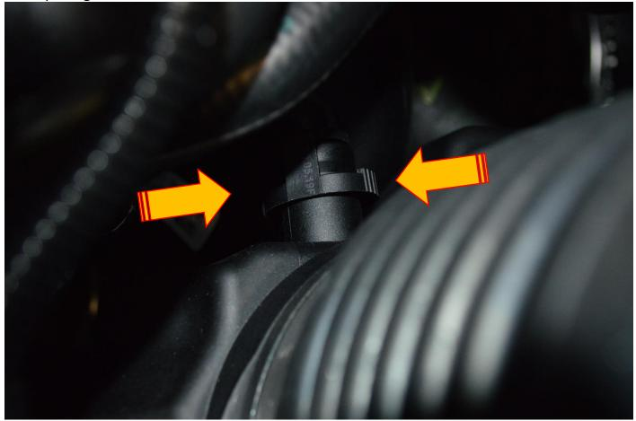
11. The inlet pipe can now be removed from situ.
