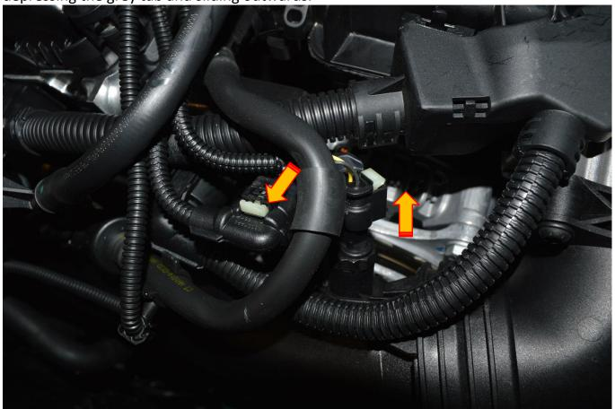
4. Remove the wiring loom from the airbox again by depressing the grey tab and sliding outwards.
