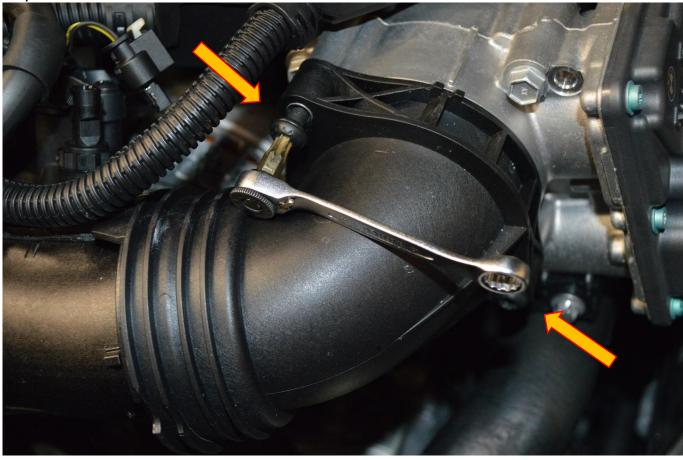
8. Pull out the retaining clip from the coupler that connects to the turbo.
