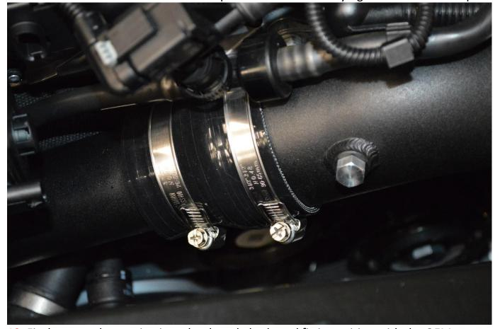
19. Fit the upper boost pipe into the throttle body and fix in position with the OEM fasteners.
