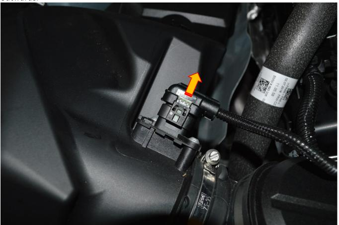
5. Using a 7mm hose clamp drive undo the hose clamp that holds the inlet pipe to the airbox.
